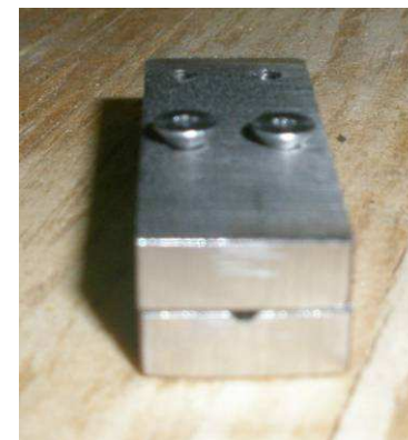
High speed wear simulation test on a grinder (wear probe rubbing against spinning abrasive surface).
