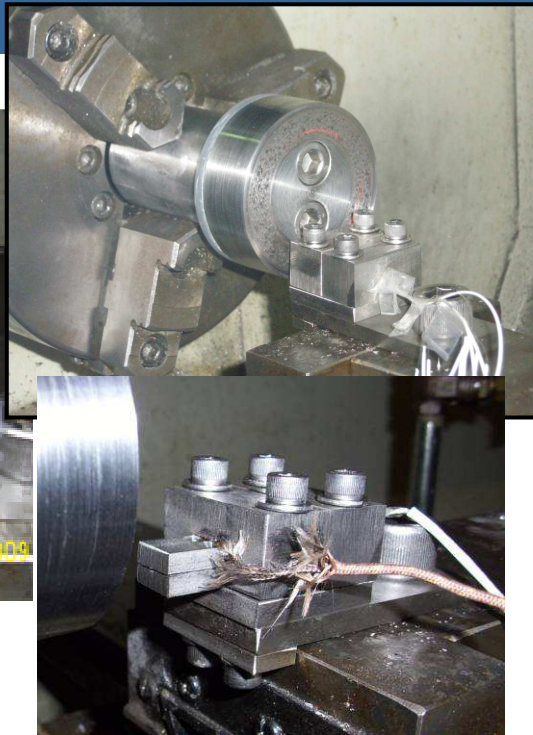
High speed wear simulation test on a lathe (wear probe rubbing against spinning metallic surface).
